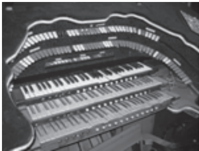
The Iowa Theatre Barton console after the floodwaters receded. This console sat in water up to its solo (top) manual for several days. Damage to the instrument and the muddy residue left behind by the floodwaters is clearly evident.
