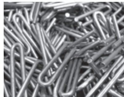
Coil cores for electric chest magnets, Organ Supply Industries (photo John Bishop)
