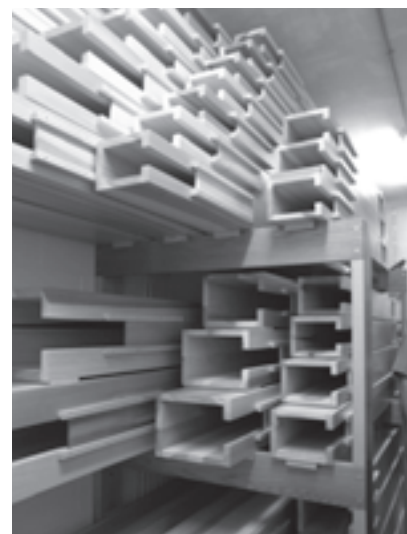
Violone and Open Wood pipes stacked in position on the roof of the organ (photo credit: Louis Patterson)
