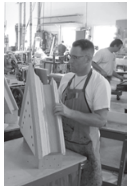
Woodworker Jon Taylor finishes capitals
