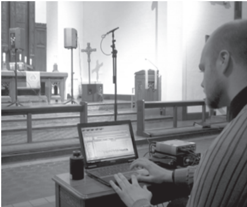
Eric Wolfram conducting acoustical testing with computer, microphones, speakers, and sound-generating equipment
