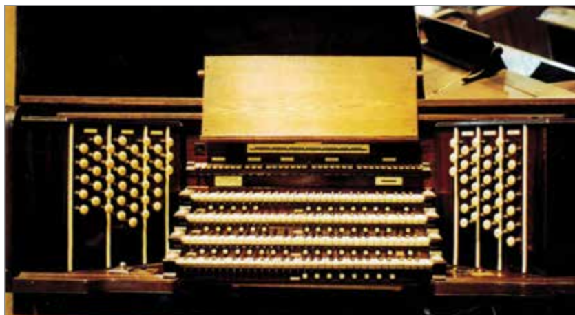
The 1928 M. P. Möller console. The horizontal bar below the music rack and above the coupler tablets sets the combination action. A metal tab is slid left or right to the proper piston and pushed to set the desired button.
