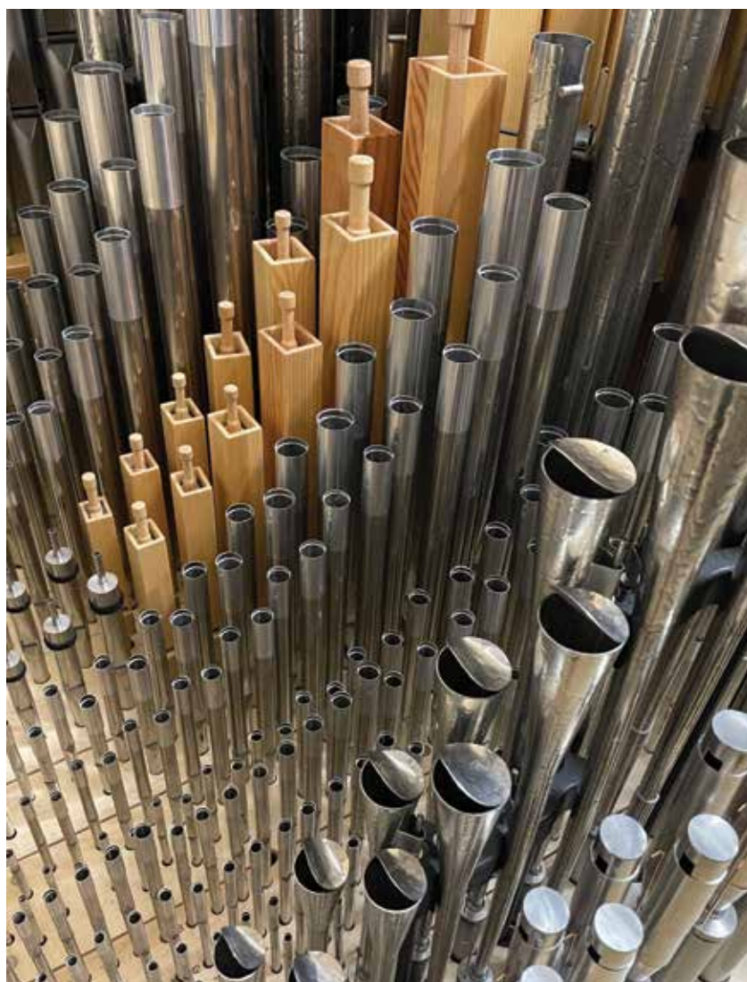
Pipework within the Swell division, including the 8' Oboe and the 8' Vox Humana in the lower right corner (photo credit: Andrew Forrest / Létourneau Pipe Organs)
