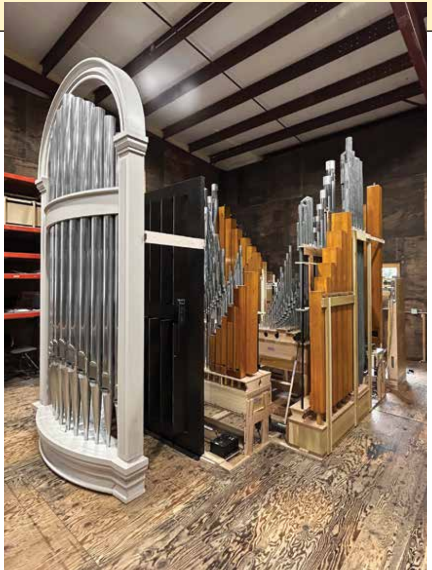
Nave division set up in workshop for testing
