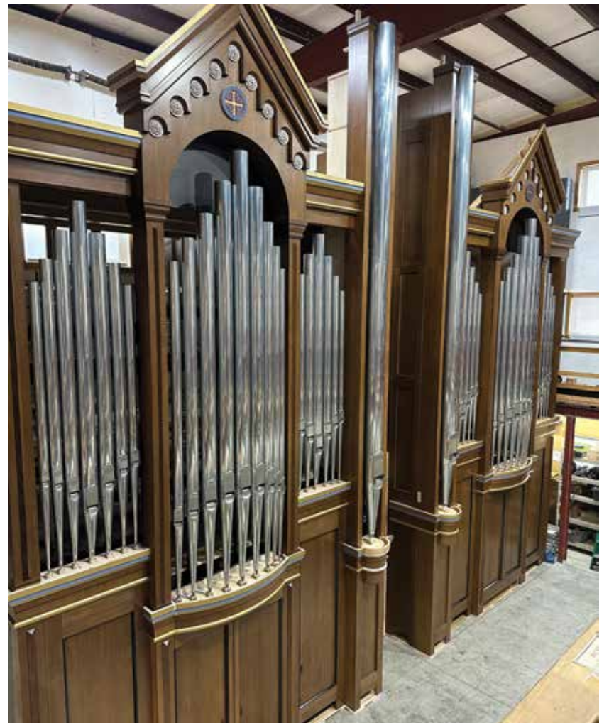
Leftmost (Choir & expressive Great) and rightmost (Swell) casework assembled in workshop for testing
