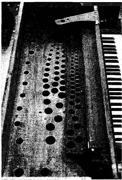
View from above of the rackboard and chest. The brace at the far end provides a bearing for the Principal stop action as well as racking for a single stopped bass pipe.
