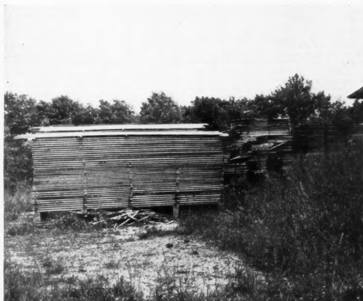
Lumber being dried and seasoned prior to movement to dry kiln.
