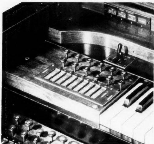
The detachable pedal unit consists of a 32-note console and radiating clavier. It is built according to A. G. O. standard dimensions. The sharp keys are molded Bakelite and the natural keys maple with a wear-resisting finish. The four toe pistons to the left of the expression pedals enable the organist to use any desired pedal quality. The two expression pedals independently affect their respective manuals. Each operates over the wide range for which the Hammond is noted—the most effective dynamic control known to music.
