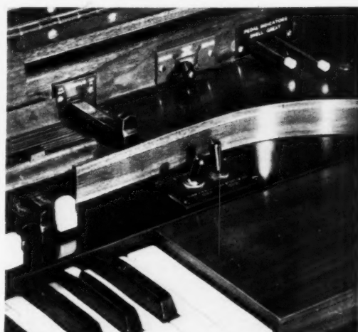
The detachable pedal unit consists of a 32-note console and radiating clavier. It is built according to A. G. O. standard dimensions. The sharp keys are molded Bakelite and the natural keys maple with a wear-resisting finish. The four toe pistons to the left of the expression pedals enable the organist to use any desired pedal quality. The two expression pedals independently affect their respective manuals. Each operates over the wide range for which the Hammond is noted—the most effective dynamic control known to music.
