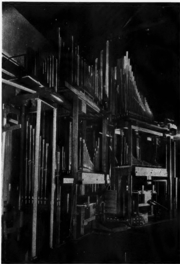
NOW BUILDING PORTION OF DIAPASON AND REED CHORUSES OF THE GREAT OF CLAREMONT COLLEGE ORGAN IN ERECTING ROOM OF FACTORY AT BRATTLEBORO.
