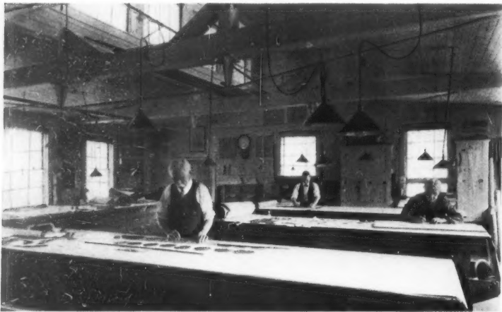
Every organ is first built on paper in the drafting room. In this department Mr. Haskell, with his assistants, works out the scales of the various stops and the layout of the different sections of each installation. Every detail of the case is designed. The console and the arrangement of its accessories are planned. From this room detailed instructions on how to construct the various parts are sent out to a score of departments. From the drawings and records in this drafting room it is possible to duplicate exactly any organ ever built by the company.
