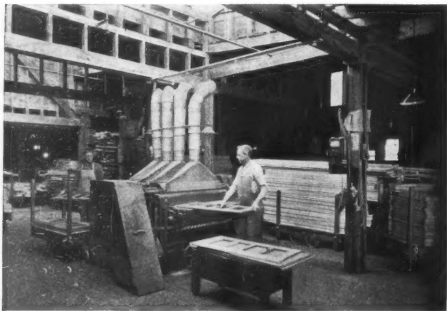
This self-feeding sanding machine is one of the many modern machines in the "mill," where the lumber is sawed and planed into approximate size for framework, chests, wood pipes and cases.
