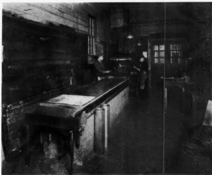
Certain tone qualities require a special mixture of metals which are cast in this room. Few, if any, other organ builders are equipped to do this work in their own factory. The foreman of this department started to learn his trade fifty-two years ago.
