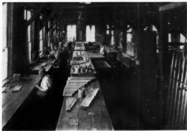
On this floor and the floor above, all the metal pipes are cut and formed out of sheet metal. At the other end of this floor is located the large annealing oven in which certain kinds of metal must be treated for five or six hours before they can be worked.
