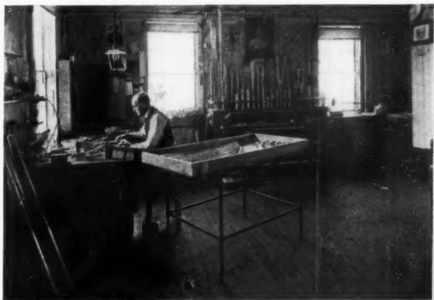
Every "voicer" has a room of his own with his own workbench and testing machine. This man specializes on reed stops. Starting with brass tubing and brass sheets he makes even the echalotes and tongues and mounts them on the block.
