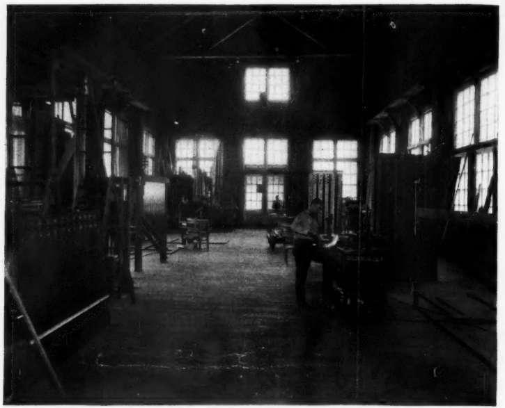
One of the two large rooms composing the "erection shop," in which every organ is completely set up and actually played and tested before it is crated and shipped to the purchaser. Among other advantages this feature of our methods makes possible rapid installation of the organ in its final location with a minimum of confusion and interruption to the regular use of the edifice.
