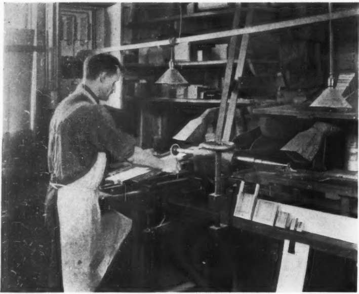
This is a special machine for cutting mouths in wood pipes and for making caps. Samples may be seen in the lower right-hand corner of the picture. It will do quickly and accurately the work of six men working with chisels and drills.
