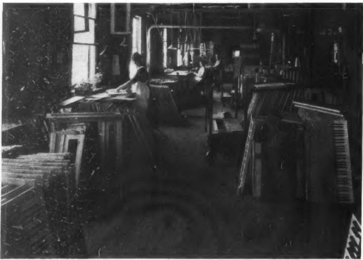
Keys and keyboards are but one of the many organ parts made in our own factory which are usually purchased from outside suppliers. Special grade sugar pine is used because of its freedom from warping. Notice the completely assembled keyboard in the lower right corner.
