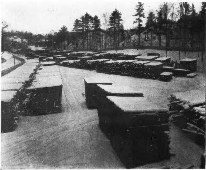
This view of the lumber yard, taken from the third floor of building No. 1, shows the large stock, which is air dried for one or two years before treatment in the dry kilns.
