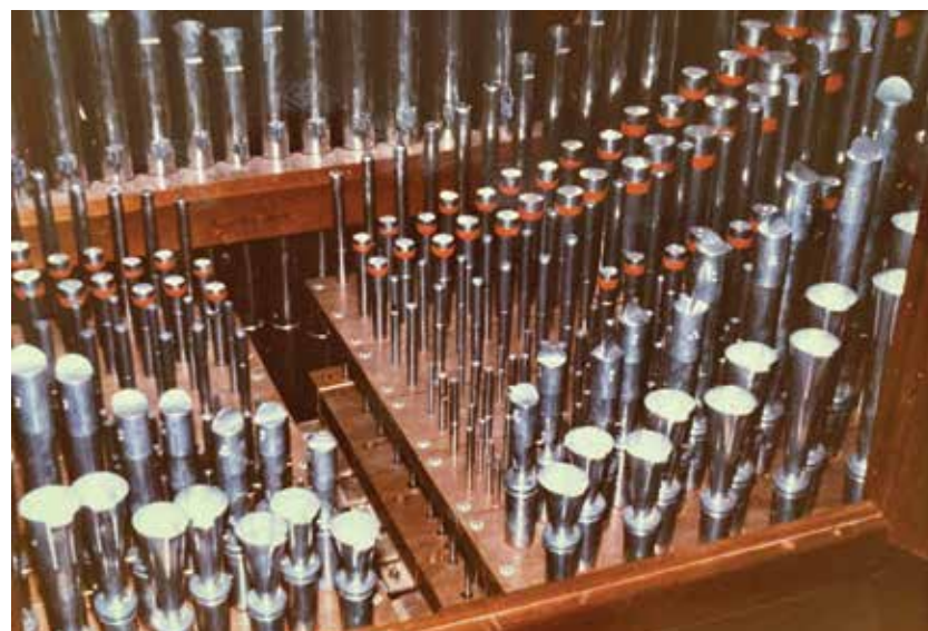
Saint Mark's Episcopal Cathedral, Seattle, Washington, 1965 D. A. Flentrop. The shallow, eleven-stop Rugwerk, looking towards the back of the 8' Prestant from the open doors at the back of the casework
