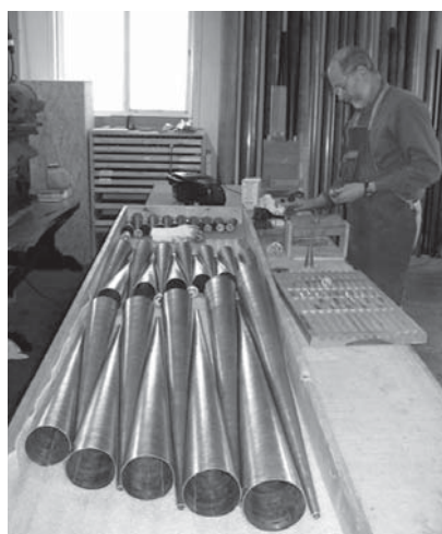
Gene Bedient solders blocks onto resonators
