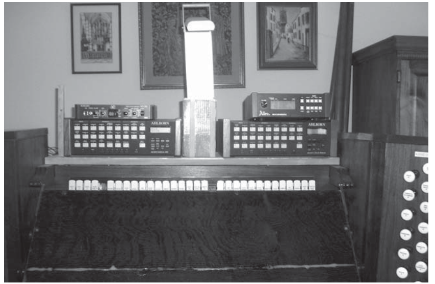
Digital modules sit on top of the console, behind the music rack
