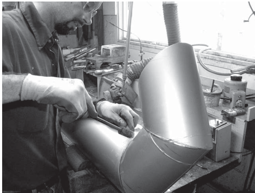
Pipemaker Rick Renko mitering the 32' Double Trombone
