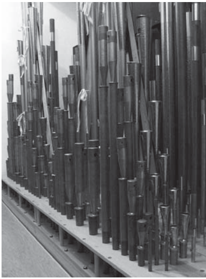
One of two soundboards in the Récit: the Voix Humaine, with its long boots, is planted in front of the Basson et Hautbois; the tin strings are in the background.
