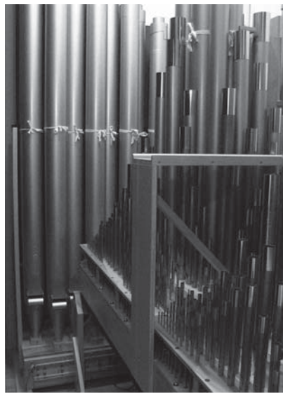
Partial view of the Grand-Orgue, showing the major third planting of the pipework. The Haskell 16' Contrebasse stands in the background.
