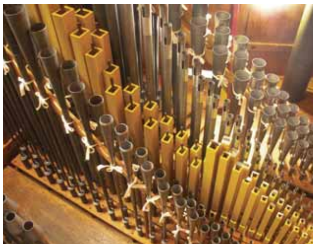
Solo division, with 8' Orchestral Oboe (1909), 8' Concert Flute, 4' Violina and the narrow 8' German Gamba. Background: 8' Tuba stop, speaking on 10" pressure (Photo credit: Andrew Forrest)
