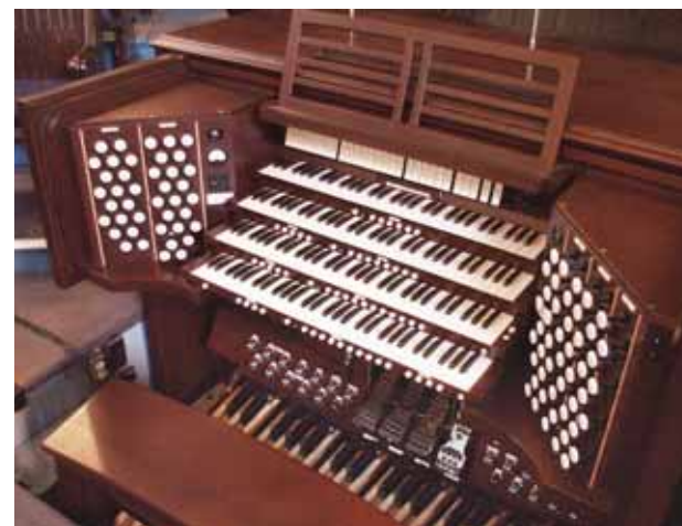
The 1938 console, rebuilt to include modern playing conveniences; elements such as the air-driven Wind and Full Organ indicators, plus the rotary crescendo indicator, were retained and restored (Photo credit: Andrew Forrest)
