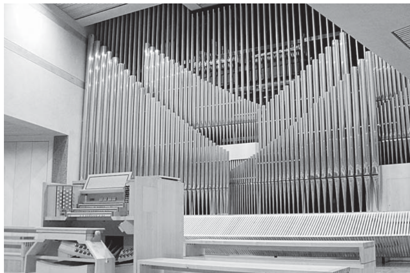
Fratelli Ruffatti three-manual, 49-rank mechanical-action organ at Chiesa del Santo Volto, Turin, Italy
