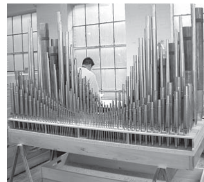
Setting pipes in one of the two new Swell windchests
