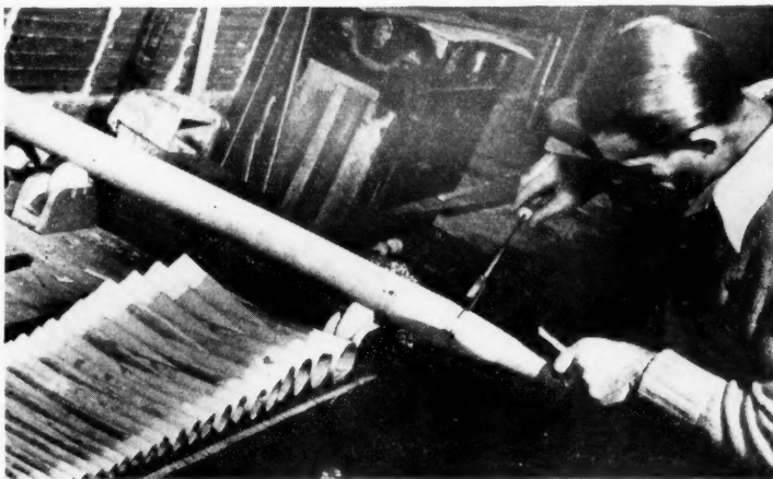
◀ FASHIONING THE METAL INTO AN ORGAN PIPE. THE CRAFTSMAN HAS BEEN OVER TWENTY-FIVE YEARS WITH THE KILGEN COMPANY. MANY OTHER PIPE MAKERS ENGAGE IN THIS WORK OF HAND FABRICATION OF ORGAN PIPES IN THE KILGEN PLANT.
