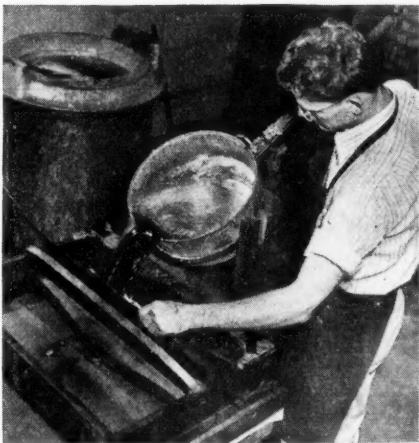
◀ POURING THE MOLTEN METAL WITH ITS PROPER PROPORTION OF TIN AND LEAD IN THE KILGEN FACTORY. IT IS THE BEGINNING OF AN ORGAN PIPE.
